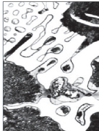
Hardness penetration of the rolls, material B10Cr
